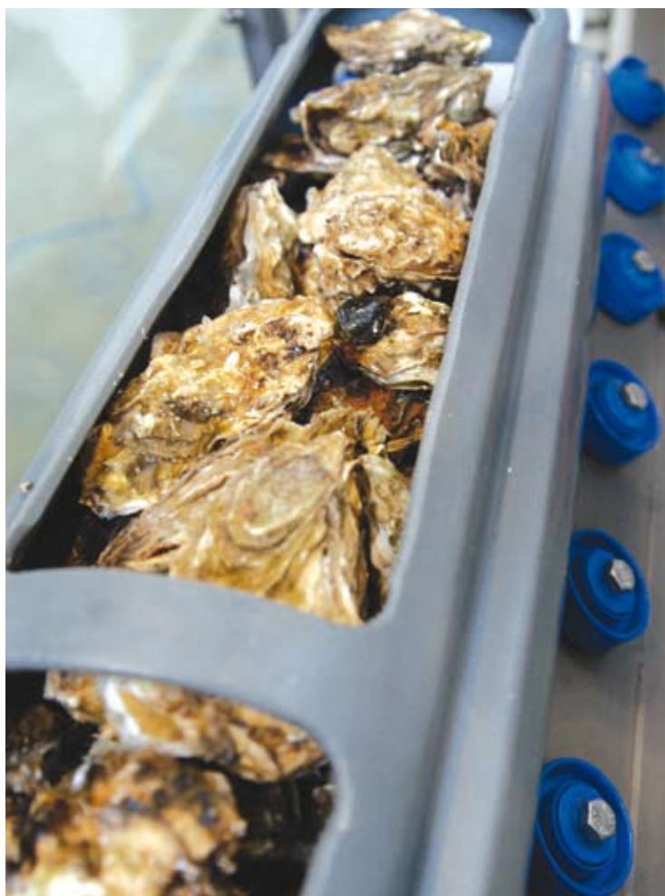
High pressure processing (HPP) causes the adductor muscle of molluscs such as oysters to open, exposing the meat for easy extraction and resulting in over 50% increase in yields.
